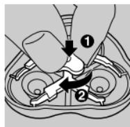
Make sure that the projections of the shaving heads fit exactly into the recesses.
