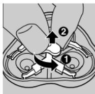
**2** Press the release button (1) to open the shaving unit (2).
